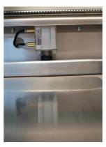
Pneumatic clamping of print frame with thickness up to 40 mm.
